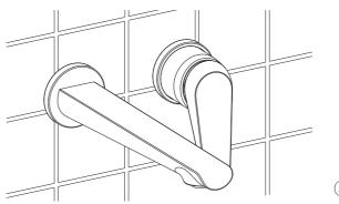
The illustration shown is the correct position of the spout and handle when the installation is completed.
